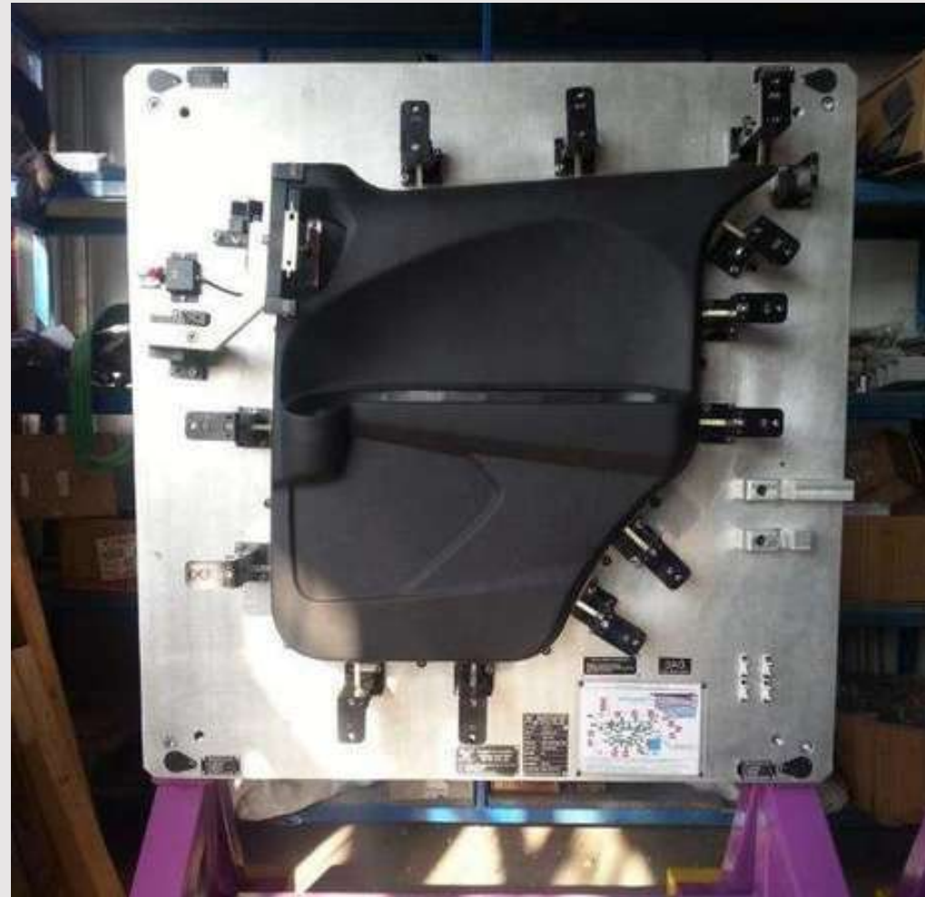
Dash Board Checking Fixture with Cameras and Pokeyoke
