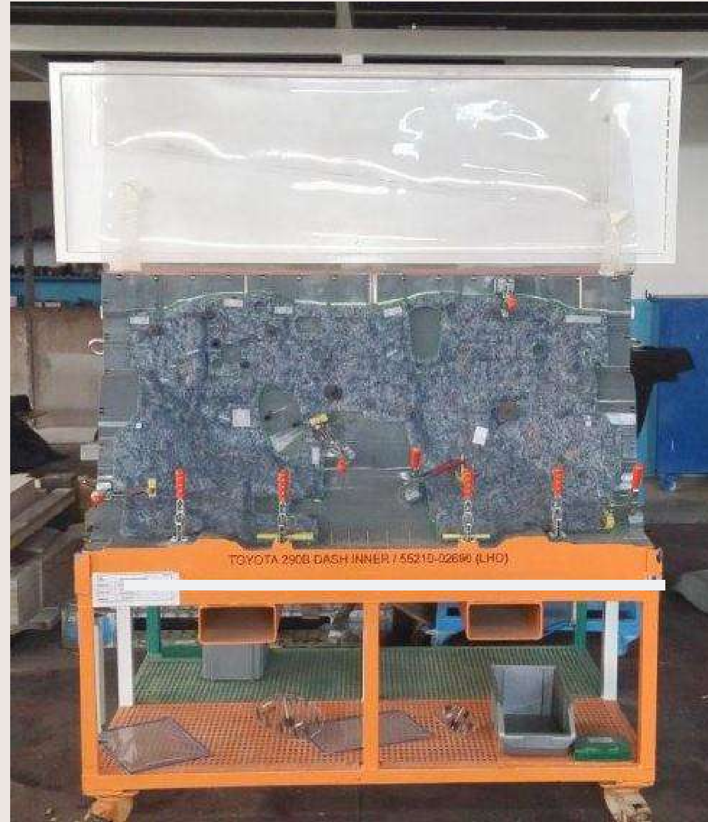
Cut Dash Inner Felt is on the checking fixture made by Maksimum Makine
