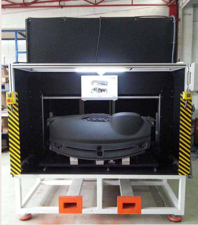
Dash Board Checking Fixture with Cameras
